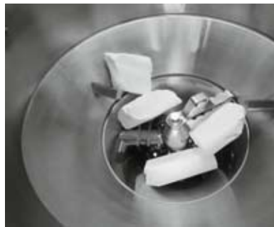
Blocks as large as 60 cm are introduced into the inlet funnel.
