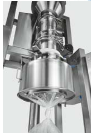
Installation for powder handling with disagglomeration, dosing and Inliner.
