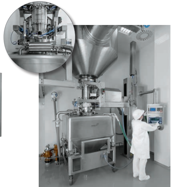
ConiWitt with High Containment valves on lift column.
